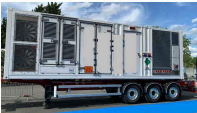
High-capacity generator set powered by renewable H2 for data centers
